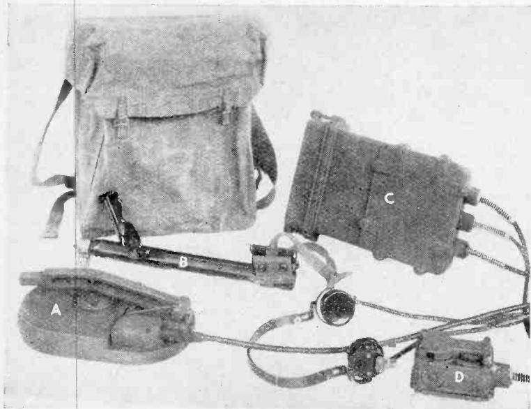
The individual units of the mine detector are shown above. The search shoe A, telescopic handle B, amplifier C and control box D are carried, together with the phones, in the canvas case.
